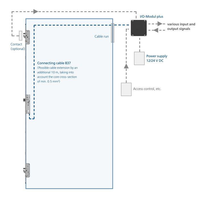
Short-term or continuous signal potentialfree for electrical lever handle activation.
