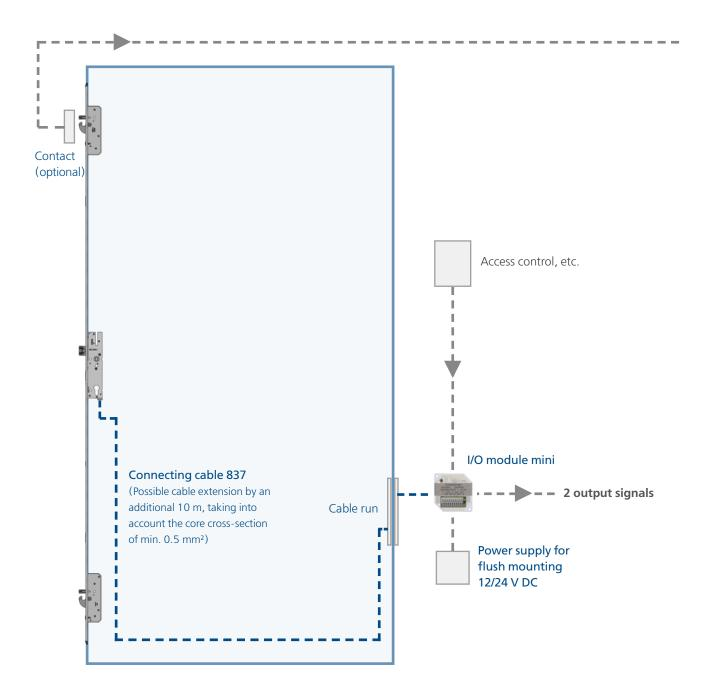
Short-term or continuous signal potential-free or 6–24 V AC/DC for electrical lever handle activation.
